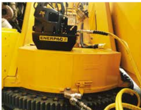
◀ Crane maintenance and assembly with S1500X wrench powered by ZU4T-Series torque pump.
